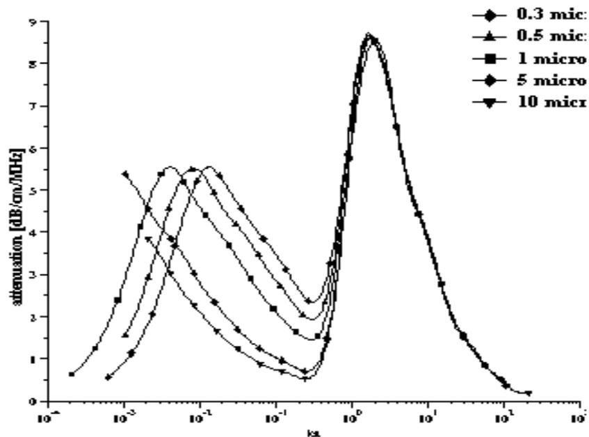
**Figure 1.1 Scattering attenuation and viscous absorption of ultrasound.**
